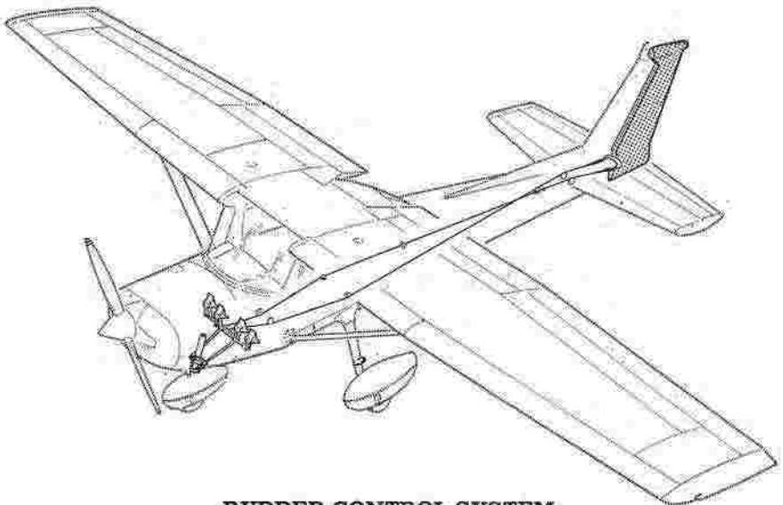
RUDDER CONTROL SYSTEM
